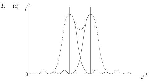
correct shape of two diffraction patterns showing central maximum and at least one secondary maximum each side of central maximum; intensity of secondary maxima no greater than one third intensity of central maxima; first minimum of one pattern coincident with central maximum of other pattern;
